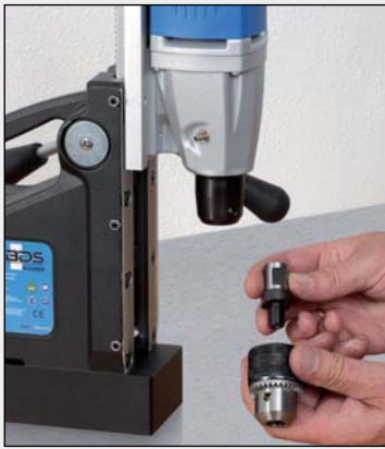
1. Connect adapter to drill chuck.
