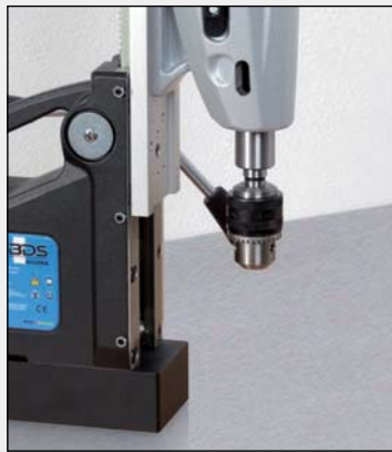
2. Place drill chuck in MT arbor.
