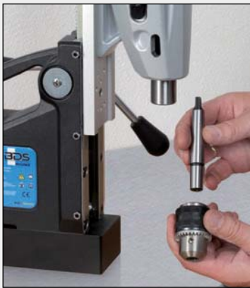
1. Connect taper drift to drill chuck.
