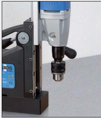
2. Place drill chuck in direct arbor.
