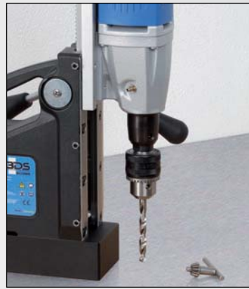
3. Ready for use with twist drill.
